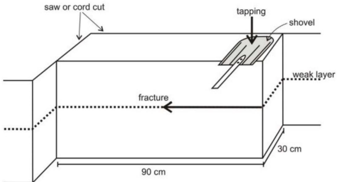
**Figure 9** *Extended column test setup.*
